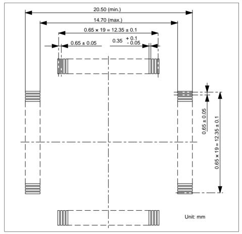
Figure 6 Recommended Dimensions for Mount Pad
